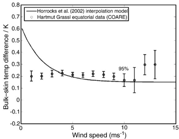
Fig. 4. Nighttime bulk minus skin SST difference plotted against measured wind speeds during the COARE campaign by Hartmut Grassl cruise in comparison with empirical formula (26).
