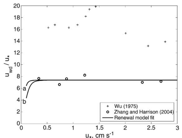
Fig. 1. Nondimensional wind-induced surface current in the laboratory tank as a function of wind friction velocity derived from surface drifters (Wu, 1975) and infrared imaging (Zhang and Harrison, 2004) in comparison with the renewal model at  $A_0 = 7.4$  for two surface cooling rates: (a)  $Q_0 = 20$  W m<sup>-2</sup>, and (b)  $Q_0 = 200$  W m<sup>-2</sup>.
