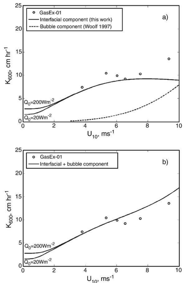
Fig. 5. (a) Comparison of the renewal type (interfacial) parameterization (20) for 2 values of the surface heat flux  $Q_0$  with direct measurements of the  $\text{CO}_2$  transfer velocity during *GasEx-2001* (Hare et al., 2004). Woolf's (1997) parameterization of the bubble-mediated component for clean bubbles is shown with a dashed line. (b) Sum of the interfacial and bubble mediated parameterizations in comparison with the *GasEx-2001* data.
