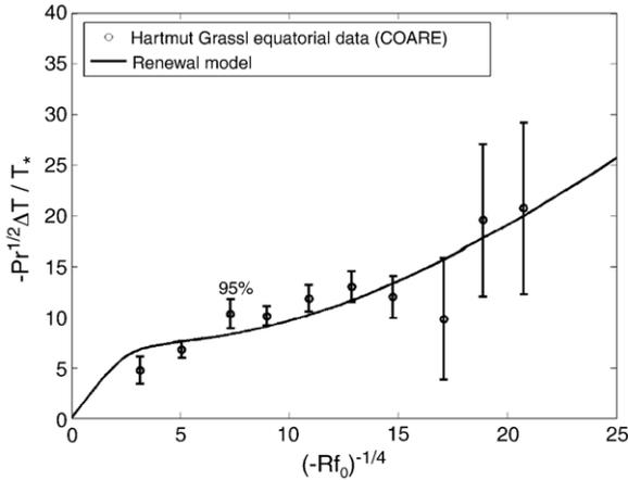
Fig. 2. Nighttime cool skin data of Hartmut Grassl obtained in the western equatorial Pacific during COARE in comparison with renewal model for developed seas ( $A_w=15$ ).
