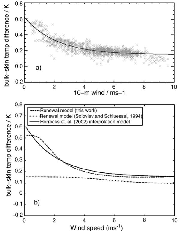
Fig. 3. (a) Nighttime bulk minus skin SST difference plotted against measured wind speeds during the R/V *Mirai* cruise (Horrocks et al., 2002). The curve is the best fit to empirical formula (26). (b) Three different models of the cools skin.
